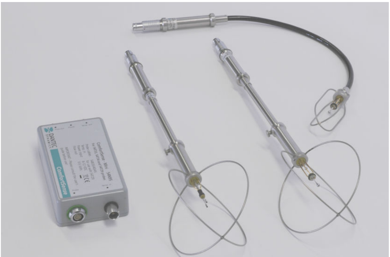
Velocity and temperature probes for the ComfortSense Mini
