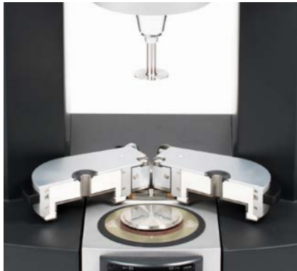
Active hood cartridge (-40°C to +150°C) environmental controller with minimized thermal gradients for plate measuring systems
