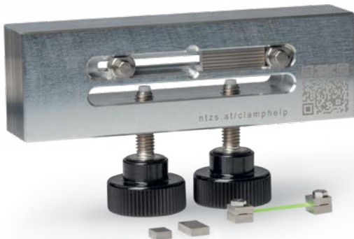
Alignment tool for sample preparation for measurements in tension mode
