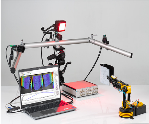
FlexDIC system used to measure the displacement of a quasi-static bending test. Components of the FlexDIC system.
