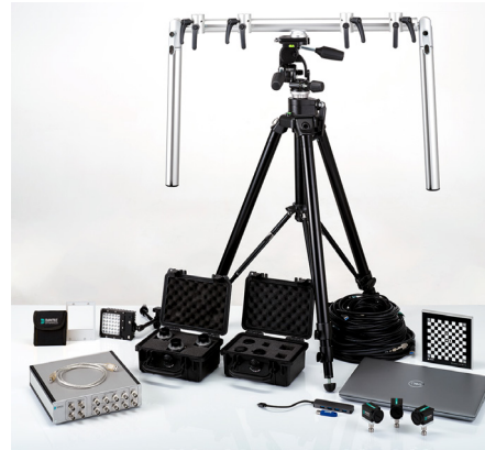
FlexDIC system used to measure the displacement of a quasi-static bending test. Components of the FlexDIC system.
