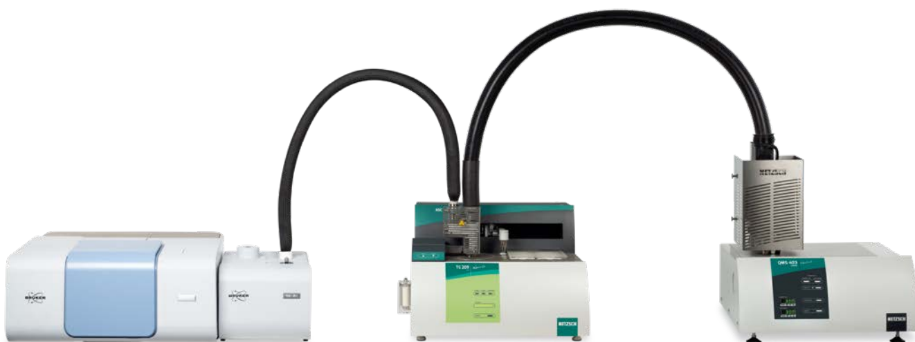
TG 209 F1 Nevio simultaneously coupled to an FT-IR (Bruker INVENIO with external gas cell) and MS (QMS 403 Aeolos Quadro)
