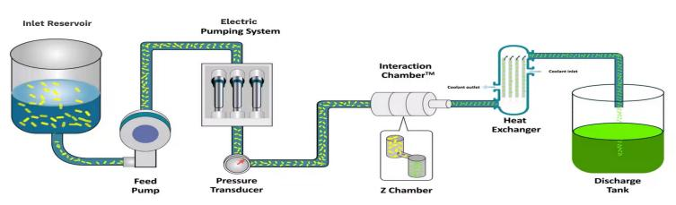
Product enters the system via the inlet reservoir and is pulled into a patented sanitary electric pumping system which pushes the material through a fixed geometry Interaction Chamber™ where it experiences consistent, high shear rates and impact forces. All material receives the same treatment to achieve repeatable, reliable results. After passing through the Interaction Chamber™, the product is cooled in the heat exchanger resulting in reduced denaturing and increased yields.
