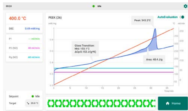
When AutoEvaluation is defined, the autonomous evaluation is available on the display after the measurement
