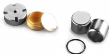
Medium-pressure crucible (right) and high-pressure crucible (left)
