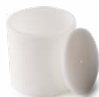
Large crucible made of Al 2 O 3 , volume 300 µl
