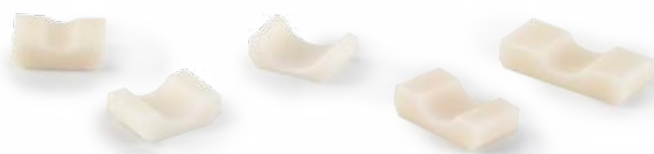
Sample-supporting kits made of alumina
