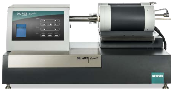
DIL 402 Expedis Supreme with SiC furnace (front) and low-temperature furnace (rear)
