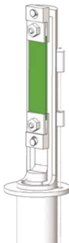
Fixture set for tension made of fused silica
