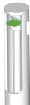
Fixture set for 3-point bending made of fused silica, bending length: 5 mm
