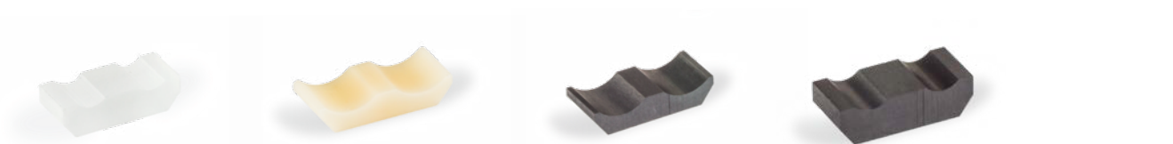
Sample-supporting kits made of fused silica, alumina and graphite for double measuring system
