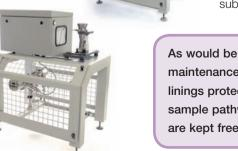
As would be expected from an industrial instrument, maintenance requirements are minimal. Ceramic linings protect critical, high-velocity areas of the sample pathway and purging ensures that windows are kept free from dust.
