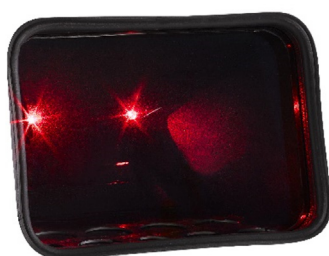
View of FlawHunter from underneath, showing a sealed area (Field-of-View) and two laser diodes.
