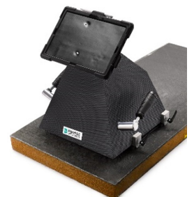
FlawHunter being used on a CFRP Laminates/Sandwich Component indicating localized impact damage and voids.
